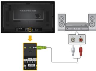
Connect a set of audio cables between the AUX L, R jacks on the AUDIO SYSTEM and [AUDIO OUT] on LCD Display.
